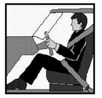
With the advent of the air bag and its deployment at about 200 mph, it is imperative that the driver and passenger be at least 11 to 12 inches away from the steering wheel or dashboard.
